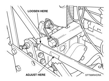
Figure 6-3. RH Steering Control Rod Adjustment
